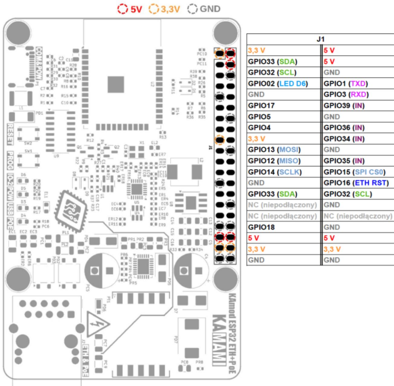
The description of the pins has also been marked on the bottom of the KAmod ESP32 board ETH+POE:
